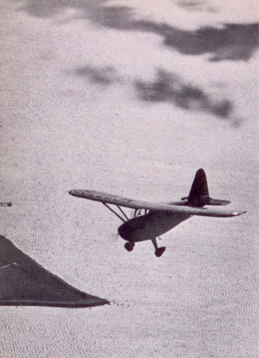
Wave action normally is a reliable guide to the wind velocity at the surface of the water. The Beaufort Scale, a guide to wind action on water, would indicate that the wind velocity was between one and three m.p.h. when this picture was taken over Long Island Sound.
